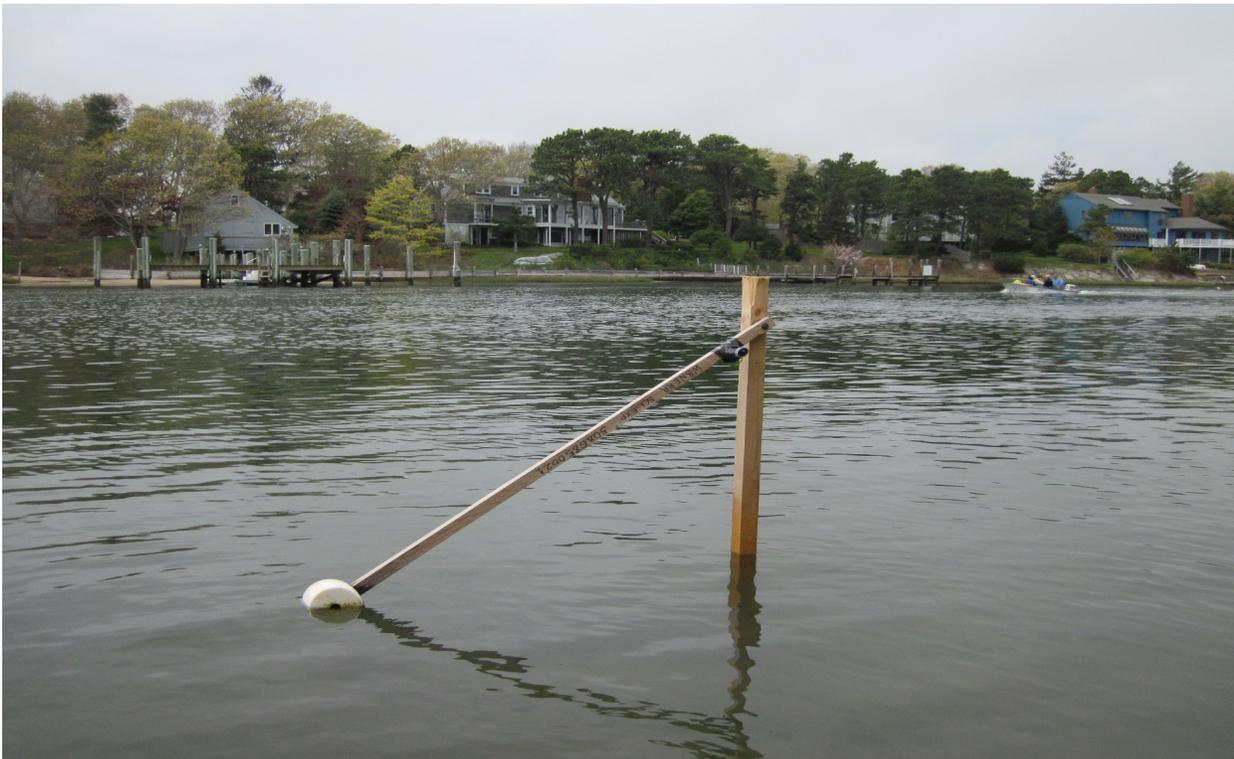
Following the test deployments some modifications were made in order to improve the instruments performance. Some issues with the bio-fouling and debris trapping were investigated. The anti-fouling paint EP2000 (made by a local company ePaint) is now used. It is a non-toxic paint approved by the EPA. During the coming winter the performance of the instruments will be analyzed with regard to the effect of icing and snow accumulation.
