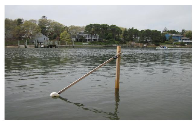
Following the test deployments some modifications were made in order to improve the instruments performance. Some issues with the bio-fouling and debris trapping were investigated. The anti-fouling paint EP2000 (made by a local company ePaint) is now used. It is a non-toxic paint approved by the EPA. During the coming winter the performance of the instruments will be analyzed with regard to the effect of icing and snow accumulation.
